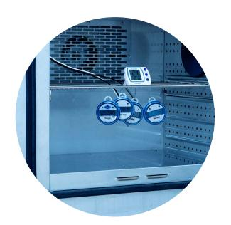
Mapping with different temperature probes (from 1 to 9 points) with variable time. (between 1 hour and 24 hours)
